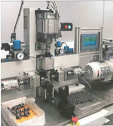
Pailton Engineering Ltd. uses this press to accurately and consistently install bearings in universal joints for steering systems. Photo courtesy BalTec (UK) Ltd.
