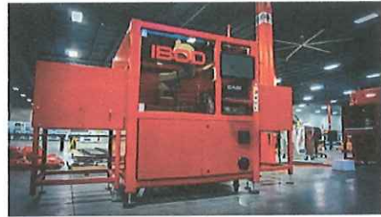
The IBOD One used by Ralawise can cut the tops off cartons at a rate of up to 450 cartons per hour. Photo courtesy TM Robotics
