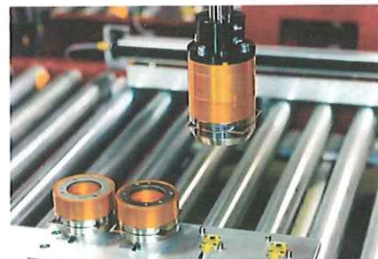
The IBOD has a blade wear monitor that tracks the life of the blades and automatically changes the blade cartridge within seconds when the blades reach the end of life threshold. Photo courtesy TM Robotics
